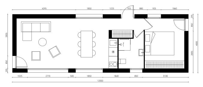
The outer dimensions: 12m x 4m x 3.95m (length/width/height) Inner dimensions: 11.5m x 3.5m x 3.1m (length/width/pitch) Total inside area: 40m2 Total outside area: 48m2
