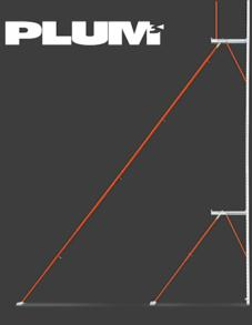
Reaching 24-feet using two Plum3 braces requires the 4-foot strongback adaptor and 3 outrigger extensions.
